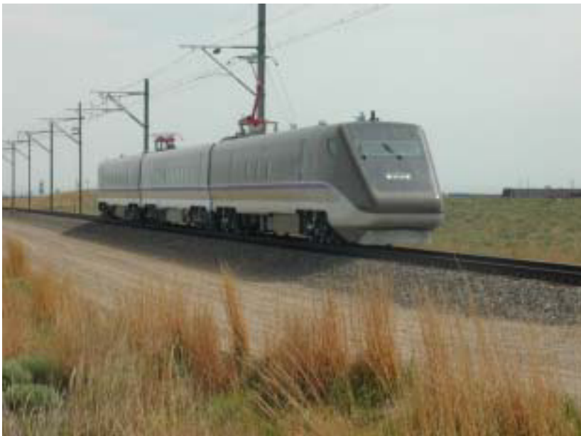
Figure 9: High-speed endurance running test at T.T.C.I. in Pueblo.
