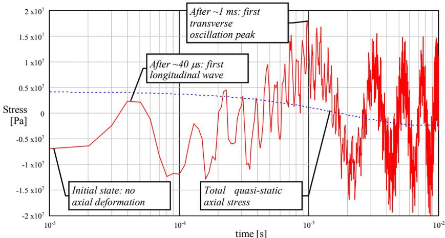
Figure 7: Total axial stress as a function of time at  $r=R$ ,  $\theta=270^\circ$ .
