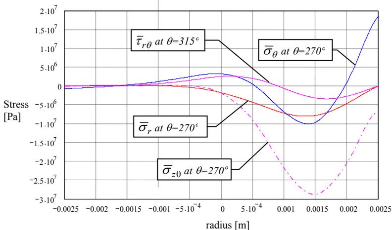
Figure 4: Quasi static stresses at  $t=t_{sp}$  as a function of radius and angle.
