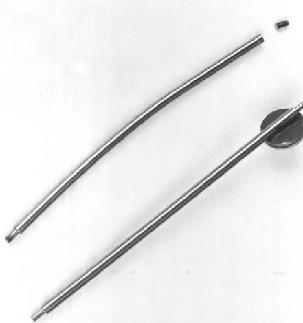
Figure 1: Example of a metallic target rod bent and broken under the effect of transverse oscillations induced by a thermal shock.
