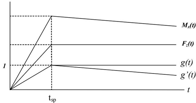
Figure 5: Equivalent dynamic excitations acting on the rod extremities.
