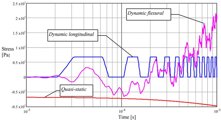
Figure 6: Quasi-static and dynamic components of axial stress at  $r=R$ ,  $\theta=270^\circ$ .
