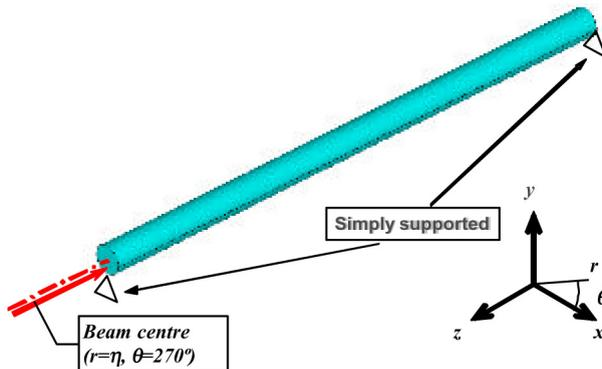
Figure 2: Target rod scheme and reference system. The rod length  $L$  is 100 mm and the radius  $R$  2.5 mm. The beam hits the rod with a 1.5 mm eccentricity and has, at its centre, a maximum energy density  $U_{Max}$  of  $8.61 \times 10^5$  J/kg. The total deposited energy  $Q_T$  is 407 J (i.e.  $4.07 \times 10^7$  W at a constant rate during 10  $\mu s$ ).
