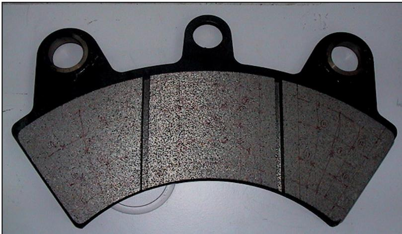
Figure 1: A Railway brake pad (non-asbestos, non-lead and semi-metallic).
