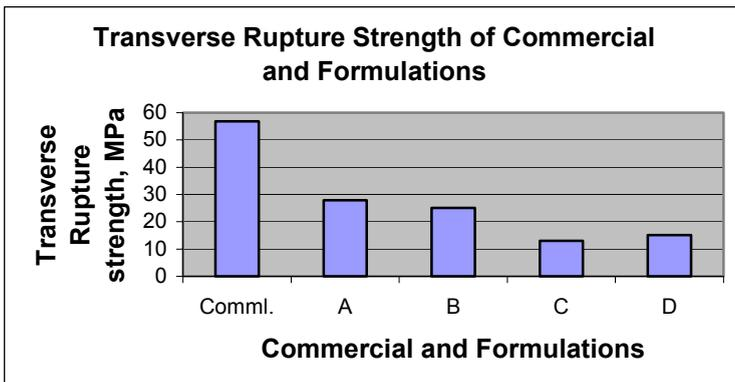
Figure 3: Transverse rupture strength of commercial and formulations.
