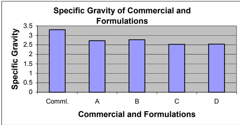
Figure 4: Specific gravity of commercial and formulations.
