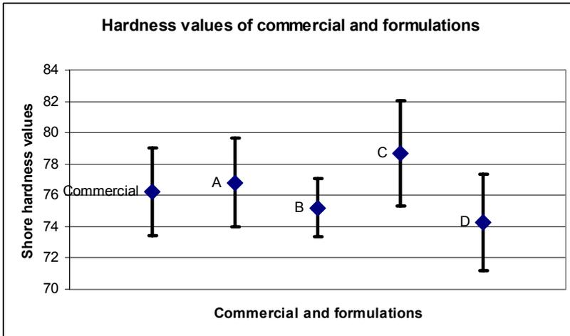
Figure 2: Shore hardness values of commercial and formulations. Data points show the mean of 15 measurements and the error bars indicate standard deviations.
