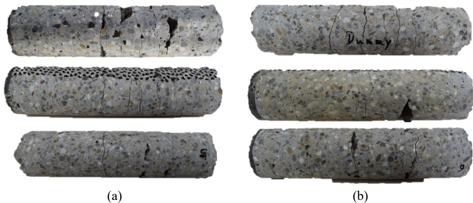
Figure 7: Fracture specimens after spalling tests under different pressures (from upper to lower rows 1.5, 1 and 0.5 bar). (a) Cylindrical projectile; and (b) Conical projectile.
