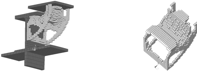
Figure 6: Optimal solution of the structural topology optimisation problem.
