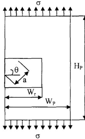
Figure 2: Geometrical model of the patched structure for the mixed mode
