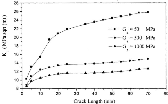
Figure 5: Effect of the adhesive shear modulus on the mode I stress intensity factor variation ( $e_a = 0.13$  mm,  $W_r = 75$  mm,  $e_r = 1.3$  mm)
