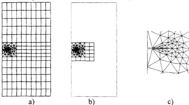
Figure 3: Typical mesh model: a) of the plate b) of the patch c) near the crack tip
