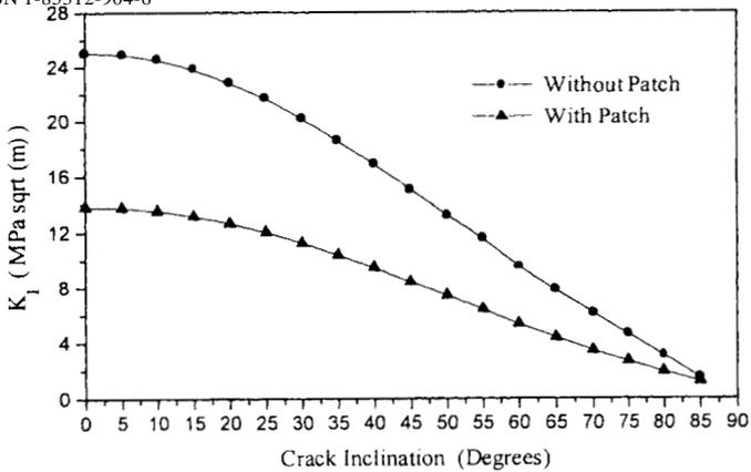
Figure 9: Comparison of the mode I stress intensity factor between patched and unpatched crack in mixed mode ( $a = 25$  mm).
