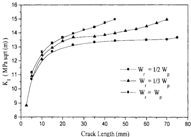
Figure 8: Effect of the patch width on the mode I stress intensity factor variation ( $G_a = 500 \text{ Mpa}$ ,  $e_a = 0.13 \text{ mm}$ ,  $e_r = 1.3 \text{ mm}$ )
