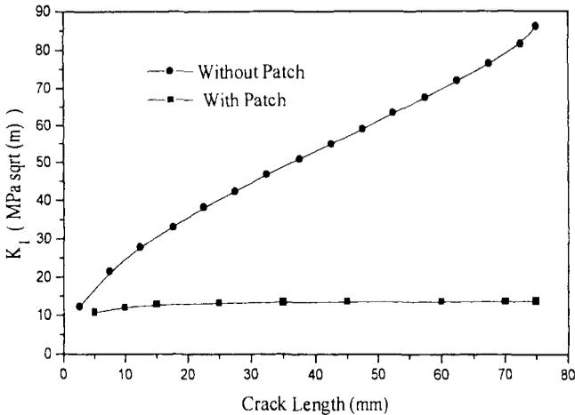
Figure 4: Comparison of the stress intensity factor between patched and unpatched cracks.
