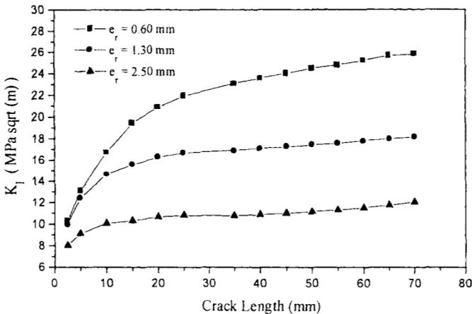
Figure 7: Effect of the patch thickness on the mode I stress intensity factor variation (  $G_a = 500$  Mpa,  $e_a = 0.13$  mm,  $W_r = 75$  mm)
