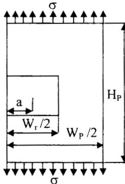
Figure 1: Geometrical model of the half of the patched structure for the mode I opening of the crack
