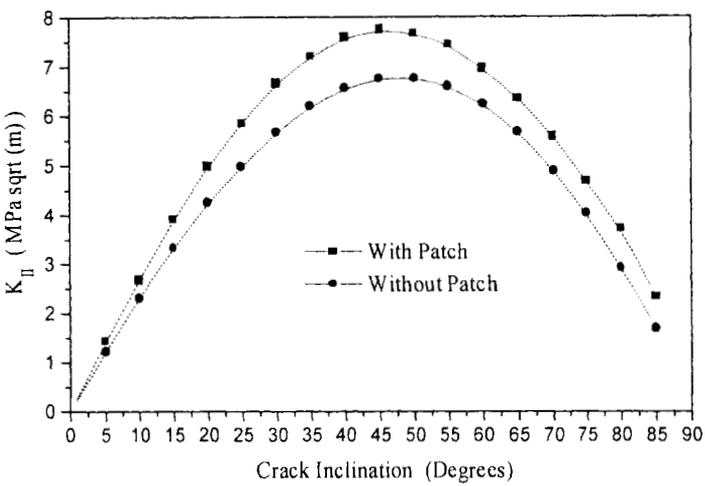
Figure 10: Comparison of the mode II stress intensity factor between patched and unpatched crack in mixed mode ( $a = 25$  mm).
