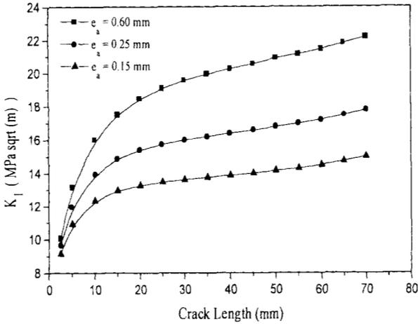
Figure 6: Effect of the adhesive thickness the mode I stress intensity factor variation (  $G_a = 500$  Mpa,  $W_r = 75$  mm,  $e_r = 1.3$  mm)
