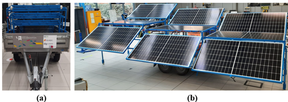
Figure 11: Final output of the FMSPS showing the system in both (a) the folded state; and (b) the unfolded state.
