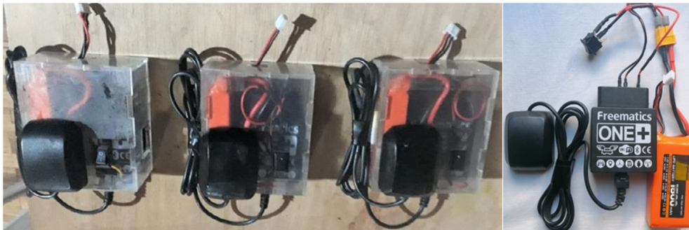
Figure 3: Freematics One+ and GPS devices used for data acquisition and Lipo battery power.
