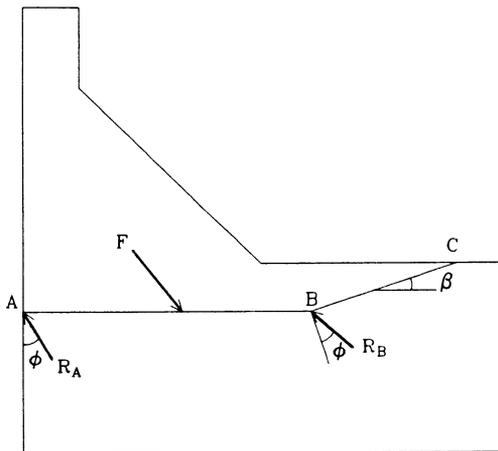
Fig. 6 - Diagram of forces assumed in analytical calculations.
