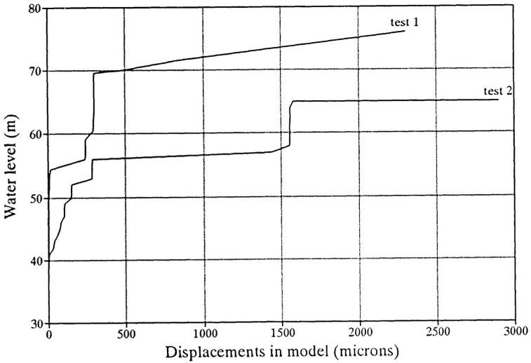
Fig. 4 - Evolution of horizontal displacement of top block with water level.
