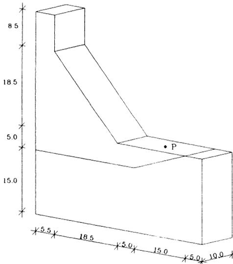
Fig. 1 - Scale model of gravity dam on jointed foundation. Dimensions in cm.
