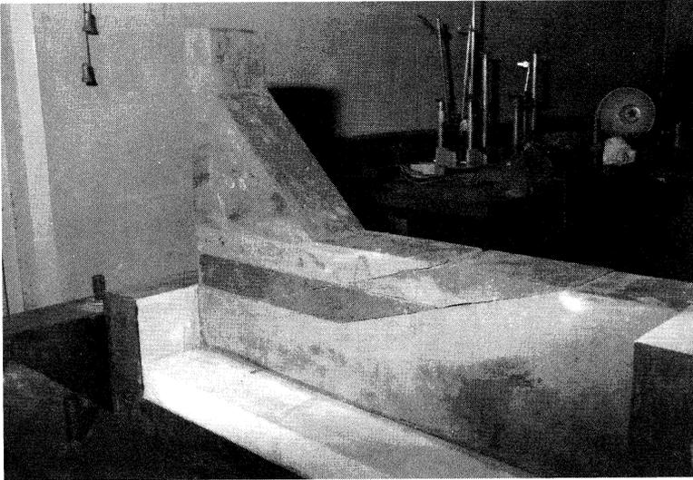
Fig. 7 - Model of gravity dam with multiple discontinuities in the foundation.
