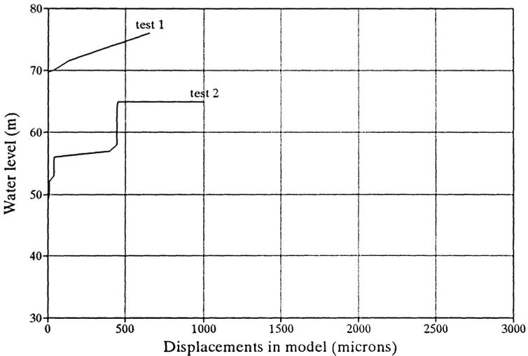
Fig. 5 - Evolution of vertical displacement of point P (in Fig. 1) with water level.
