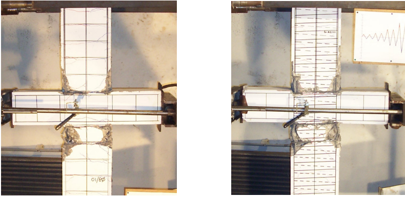
Figure 6: Final condition of specimens B1s and B1sp.
