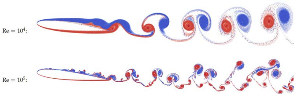
Figure 9: Vortex wake after the NACA-0012 airfoil for angle of incidence \alpha = 6^\circ at Re = 10^4 and Re = 10^5 .
