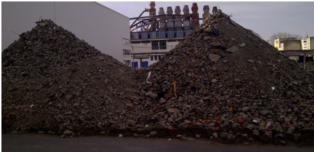
Figure 10: Filling material with impurities obtained after crushing.
