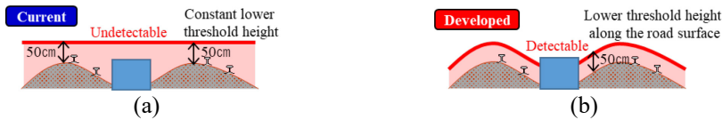
Figure 6: Map of ground surface of the level crossing. (a) Current; and (b) Developed.
