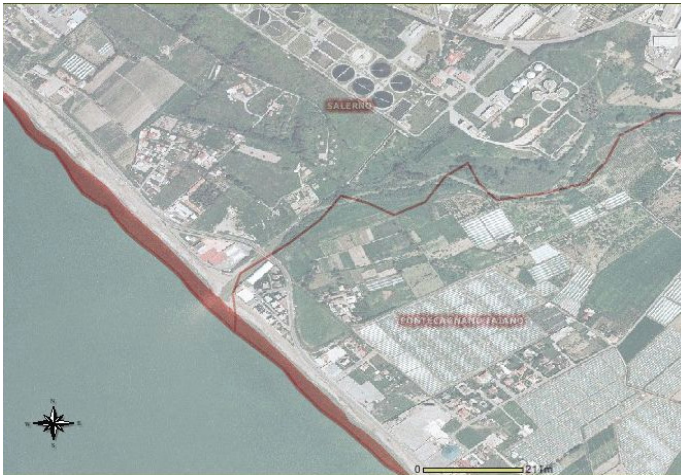
Figure 2: Long-term erosion of the Salerno coastline (the lost beach area is shown in dark grey).
